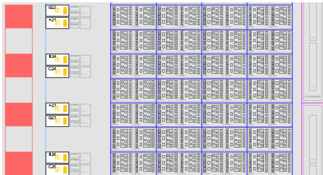
Figure 6: Zooming into the Device to view CLBs and Logic Gate Sites.
