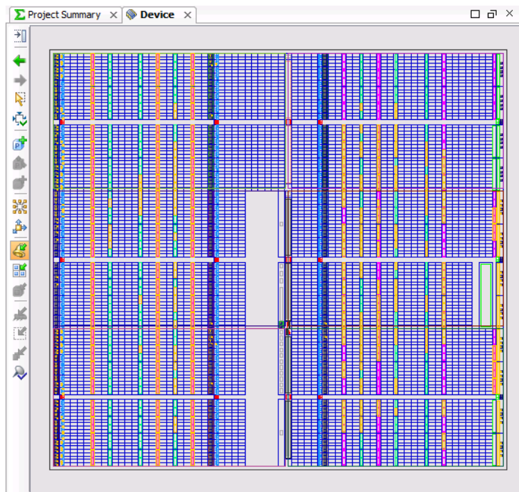
Figure 1-2: Floorplanned Logic by Hand
