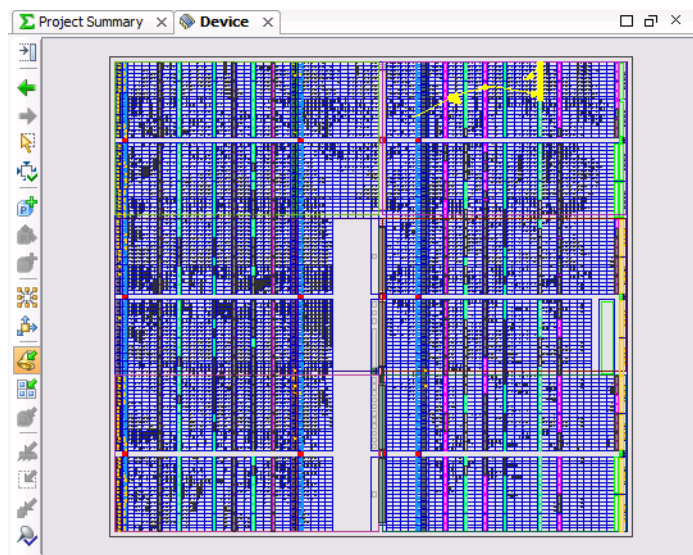
Figure 3-1: Placement of Paths Failing Timing
