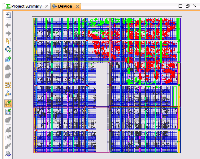
Figure 3-4: Critical and Non-Critical Parts of a usbEngine
