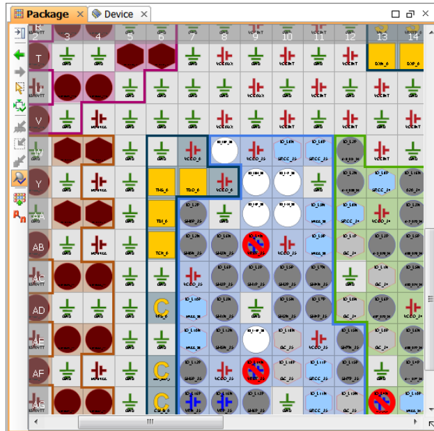
Figure 7: Examining Prohibited VREF Package Pins
