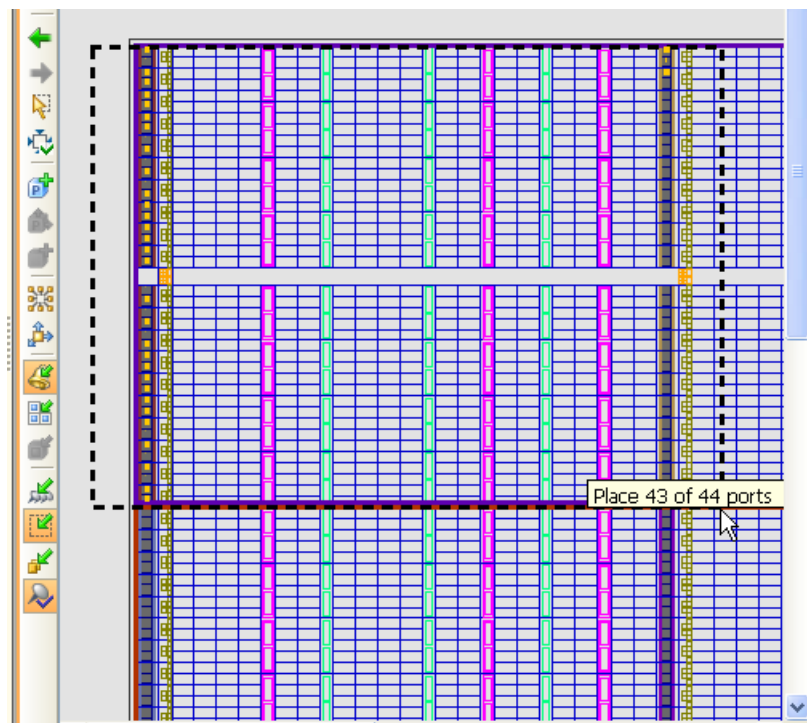
Figure 25: Placing USB1 I/O Ports in an Area
