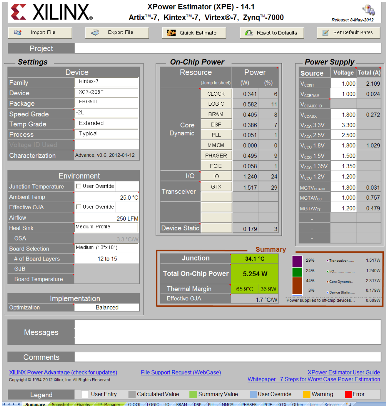
Figure 12: Summary Sheet (Kintex-7) - Adjust Settings and Display Power Results
