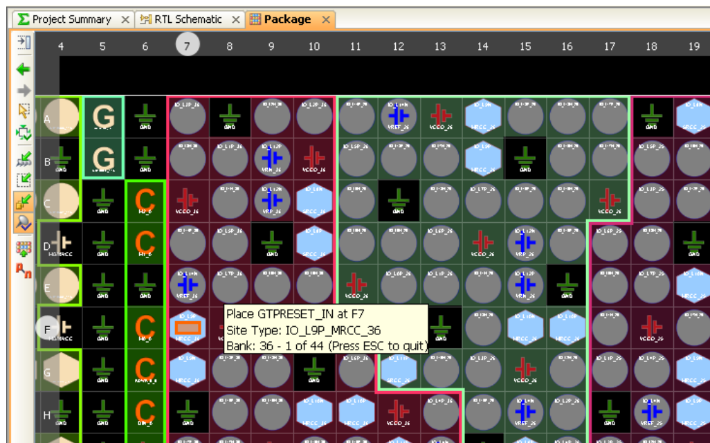
Figure 8-21: Placing I/O Ports Sequentially
