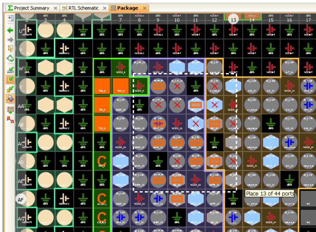
Figure 8-23: Placing I/O Ports in an Area
