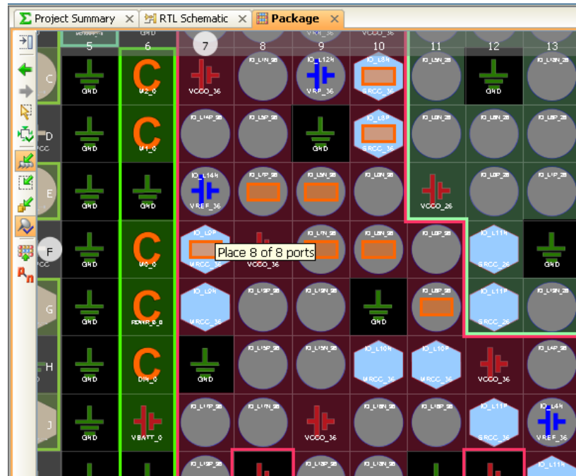
Figure 8-22: Placing I/O Ports in I/O Banks
