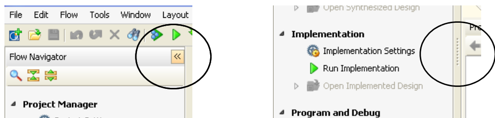
Figure 4-5: Hiding and Showing Flow Navigator
