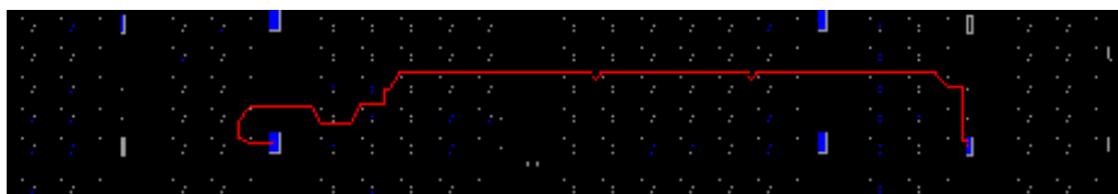
Figure 8-2: FPGA Editor Highlighted Routing
