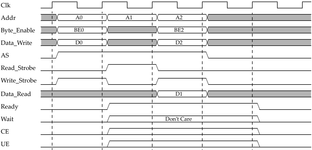
Figure 3-8: Back-to-Back Mixed Write/Read Operation, 0 Wait States
