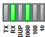
Ethernet status LEDs
