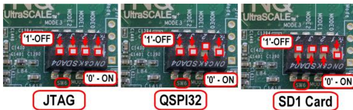
Figure 225: ZCU104 Boot Mode Switch Settings
