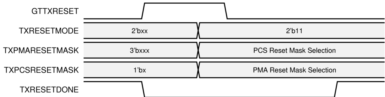
Figure 19: Transmitter Reset after GTTXRESET Pulse in Component Single Mode
