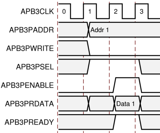
Figure 32: APB3 Read Timing
