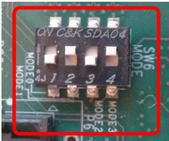
Figure 263: SD Card Boot Settings (ZCU102 Board)
