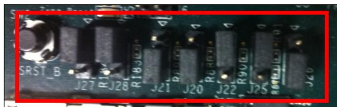
Figure 257: SD Card Boot Settings (ZC702 Board)
