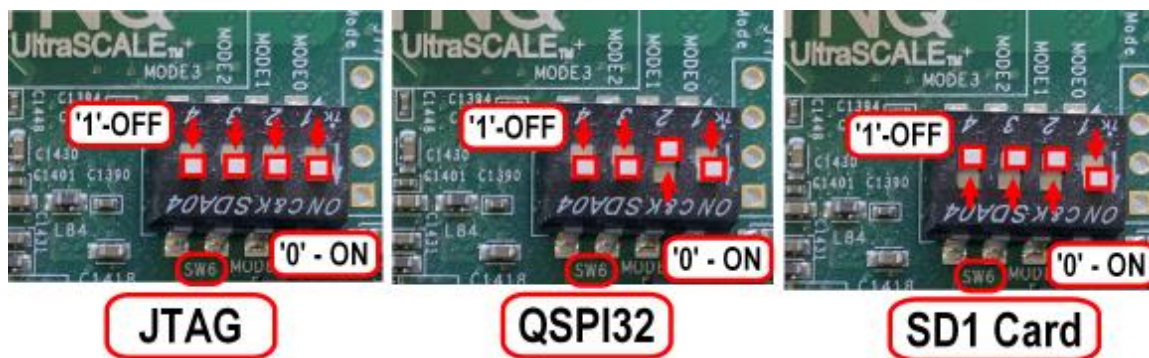
Figure 225: ZCU104 Boot Mode Switch Settings
