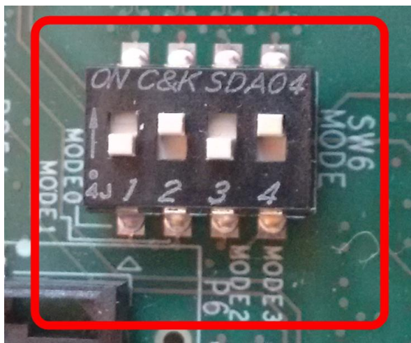
Figure 263: SD Card Boot Settings (ZCU102 Board)
