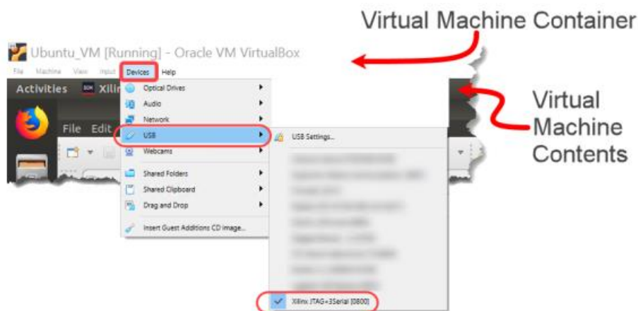
Figure 138: Selecting the Hardware Target
