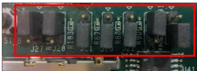
Figure 259: Flash Boot Settings (ZC702 Board)
