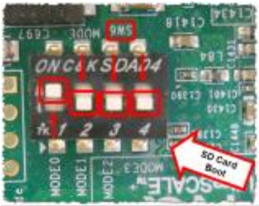
Figure 265: SD Card Boot Settings
