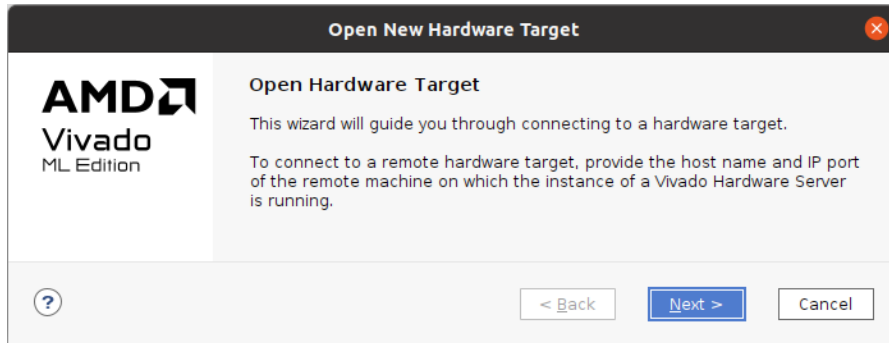
Figure 151: Opening a New Hardware Target
