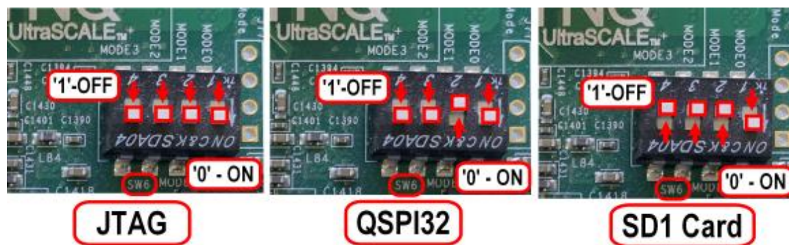
Figure 225: ZCU104 Boot Mode Switch Settings
