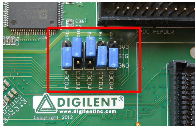
Figure 268: SD Card Boot Settings (ZedBoard)
