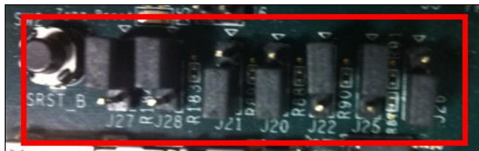
Figure 257: SD Card Boot Settings (ZC702 Board)
