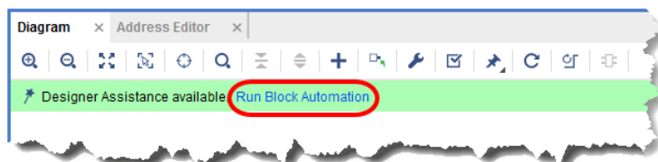
Figure 94: Designer Assistance - Block Automation (Run Connection Automation May be Absent)
