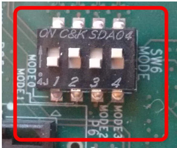
Figure 260: SD Card Boot Settings (ZCU102 Board)
