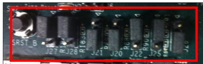
Figure 254: SD Card Boot Settings (ZC702 Board)
