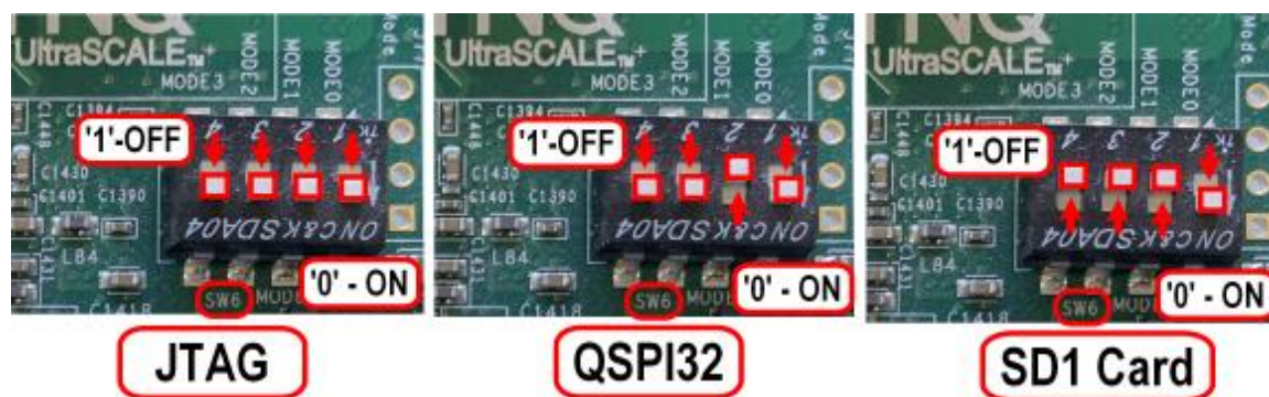
Figure 224: ZCU104 Boot Mode Switch Settings
