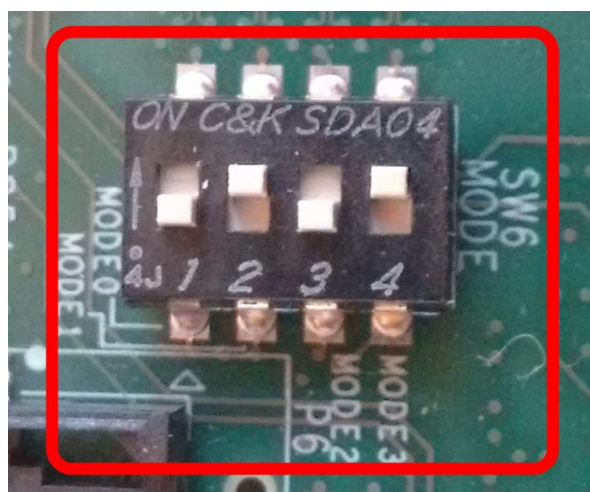
Figure 263: SD Card Boot Settings (ZCU102 Board)
