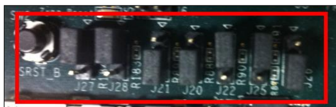
Figure 257: SD Card Boot Settings (ZC702 Board)
