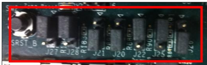
Figure 257: SD Card Boot Settings (ZC702 Board)
