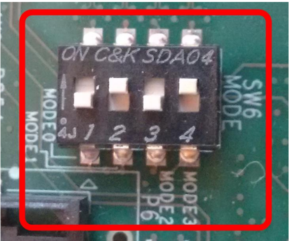
Figure 263: SD Card Boot Settings (ZCU102 Board)
