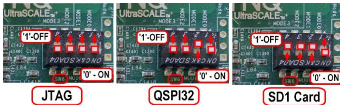
Figure 225: ZCU104 Boot Mode Switch Settings
