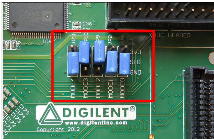
Figure 268: SD Card Boot Settings (ZedBoard)
