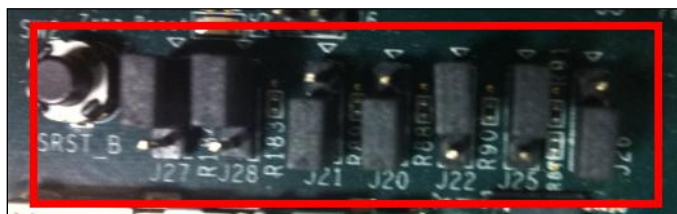
Figure 265: SD Card Boot Settings (ZC702 Board)
