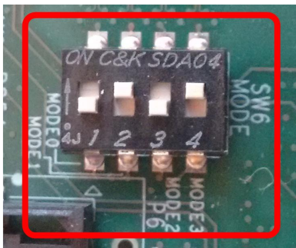
Figure 271: SD Card Boot Settings (ZCU102 Board)
