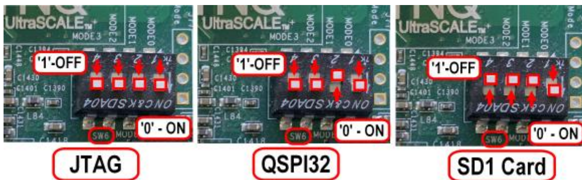
Figure 233: ZCU104 Boot Mode Switch Settings
