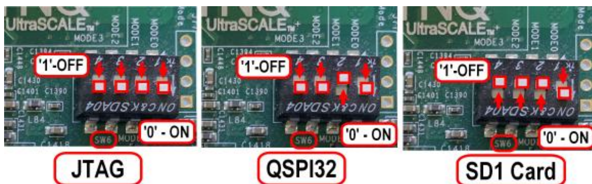
Figure 233: ZCU104 Boot Mode Switch Settings
