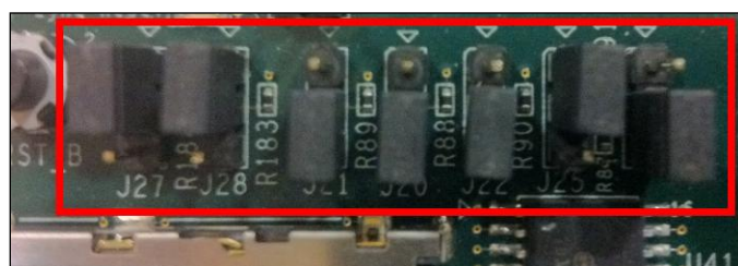
Figure 262: Flash Boot Settings (ZC702 Board)
