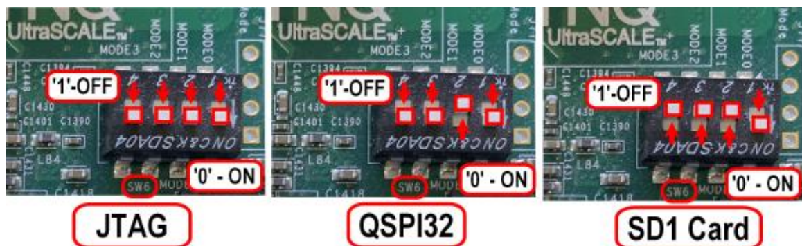
Figure 228: ZCU104 Boot Mode Switch Settings
