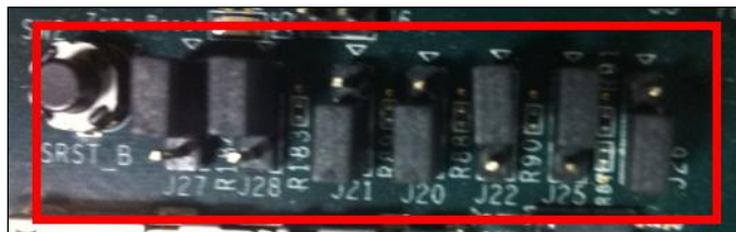
Figure 260: SD Card Boot Settings (ZC702 Board)
