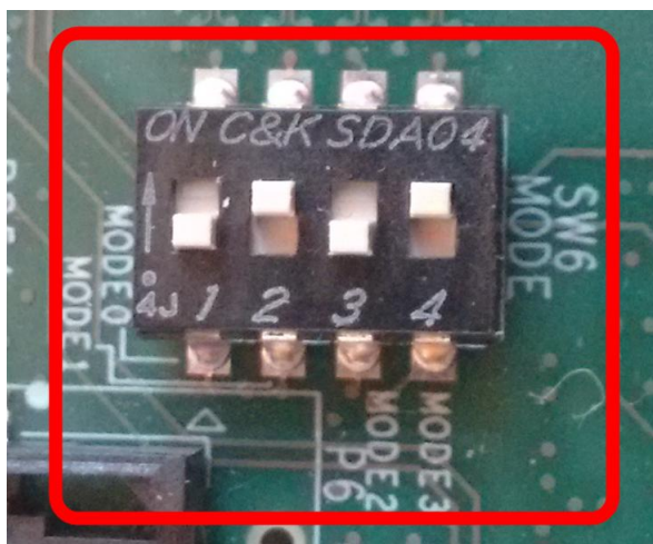
Figure 266: SD Card Boot Settings (ZCU102 Board)
