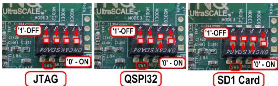
Figure 228: ZCU104 Boot Mode Switch Settings
