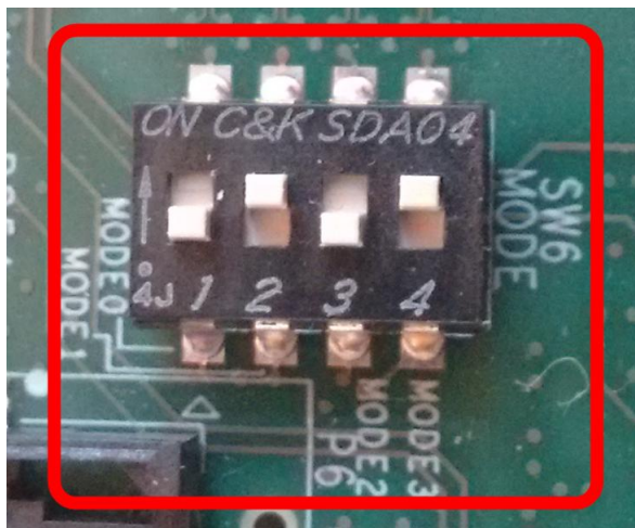
Figure 266: SD Card Boot Settings (ZCU102 Board)
