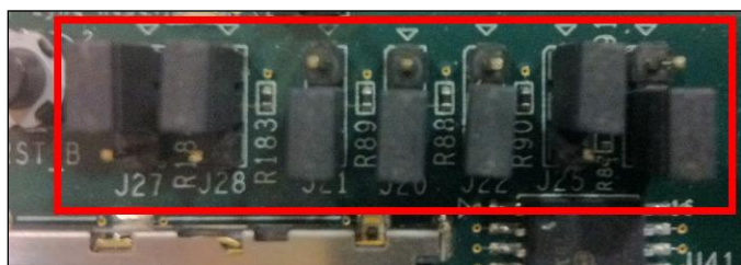
Figure 267: Flash Boot Settings (ZC702 Board)
