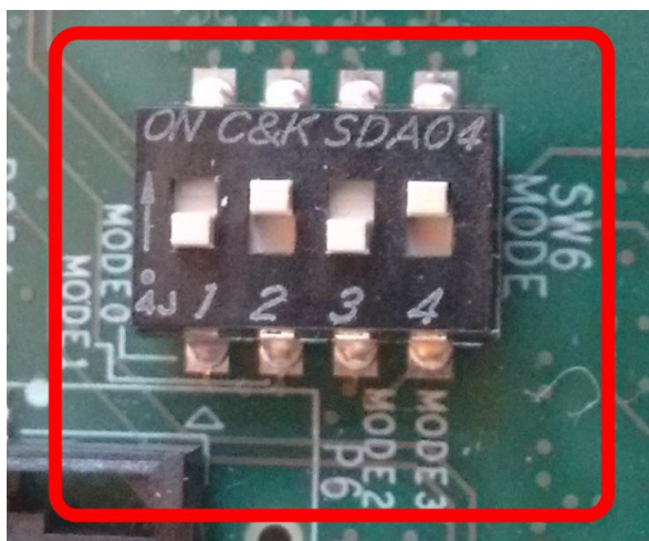
Figure 271: SD Card Boot Settings (ZCU102 Board)
