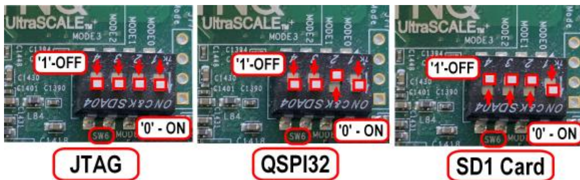
Figure 233: ZCU104 Boot Mode Switch Settings
