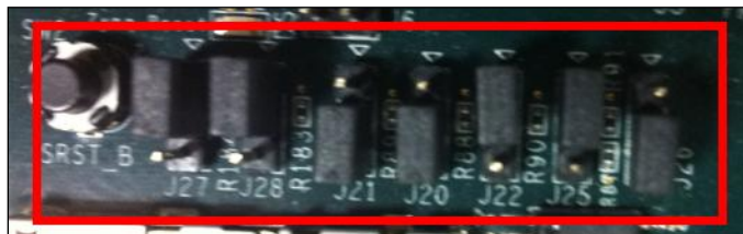
Figure 265: SD Card Boot Settings (ZC702 Board)
